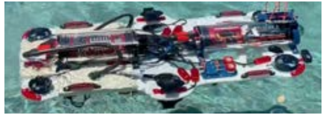
Fig. 7. Buoyancy test of Dragon with foam and its final frame constructed out of HDPE.
