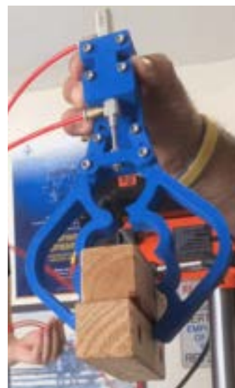
Fig. 8. Testing the grabber mechanism with a solenoid.
