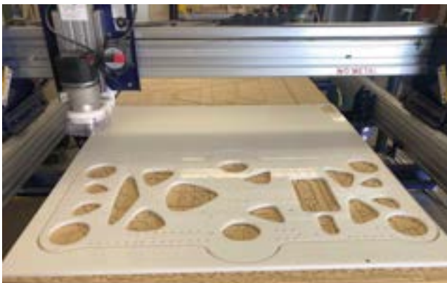
Fig. 6. HDPE frame being cut on a CNC router.
