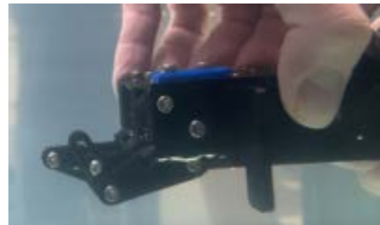
Fig. 12: Spring-loaded slot blocking launcher.
