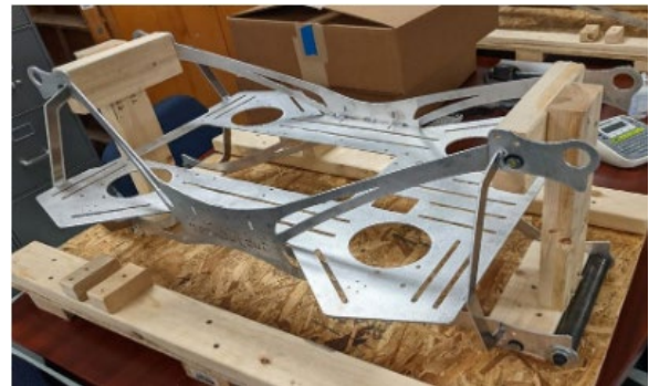
Fig. 10. SubjuGator 9 chassis. Made from 1/4" 6061-T6 plates.
