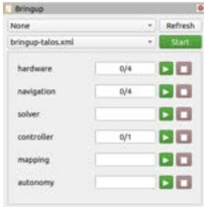
Fig. 20: The RViz bringup panel is used for remotely starting the robot. This panel allows for staging and monitoring startup of the software.
