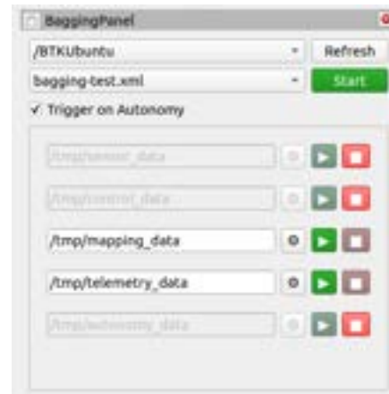
Fig. 23: The RViz bagging panel is responsible for configuring, starting, and stopping logging onboard the AUV during runs. It also can synchronize with the mission system to allow for automatic starting and stopping of logs when behaviors are executing.
