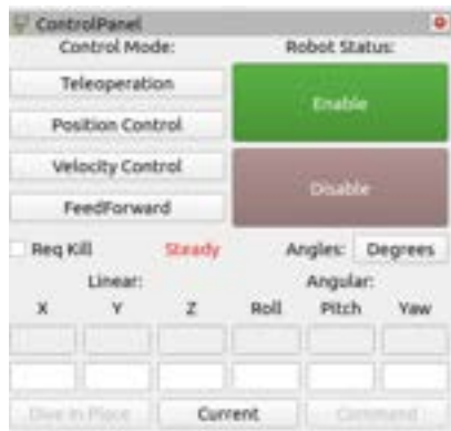
Fig. 21: The RViz control panel is used for commanding the vehicle while in the water. It allows for sending commands directly to the robot and reading out its current estimated location.
