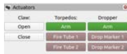
Fig. 24: The RViz actuators panel allows an operator to have direct control over the task mechanisms onboard the AUV. It also includes safety interlocks required for operation of critical systems like the torpedoes to prevent accidental discharge.
