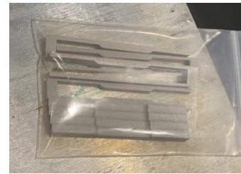
Fig. 7: Test samples cut from the stock of mystery aluminum
