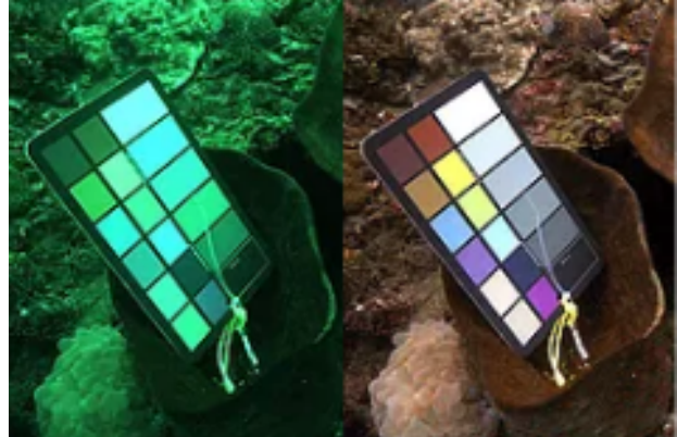
Fig. 3. Non-color corrected image on the left and image with Sea-Thru algorithm applied on the right
