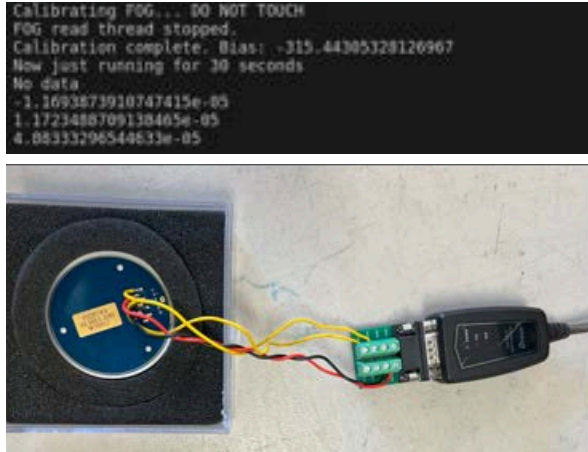
Fig. 6. Configuration of unit test for our FOG. By moving the physical FOG and looking at our outputs, we were able to verify that the FOG had an error of between 1^\circ to 2^\circ .
