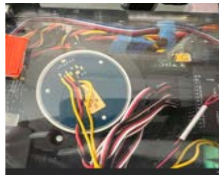
Fig. 3. FOG inside Onyx's electronics enclosure.
