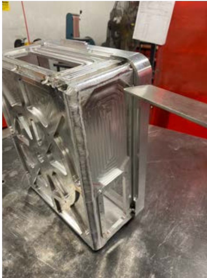
Figure 29: Weld Joint Finished
