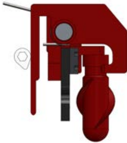
(a) Cam before it has engaged with the Dropper Restraining Finger
