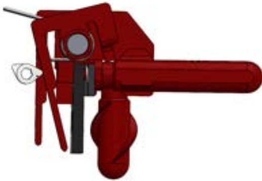
(c) Cam after it has lifted the Torpedo Restraining Finger to its maximum deflection
