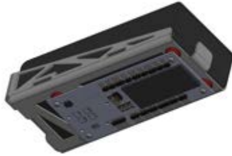
Figure 25: Tray with Battery Board and Battery
