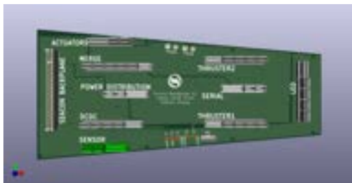
Fig 5. 3D model of updated backplane on Polaris.
