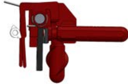
(b) Cam after it has started engaging with the Torpedo Restraining Finger
