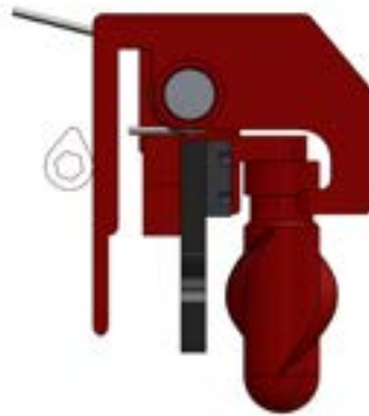
(d) Cam after it has returned the Dropper Restraining Finger to the original position
