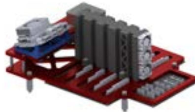
Fig 3. Sirius racks, featuring 3D printed components.
