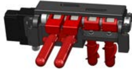
Fig 2. Sirius torpedoes and droppers system.
