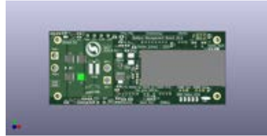
Fig 6. 3D model of BMB board located in battery pods.
