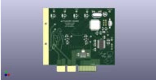
Fig 8. 3D model of updated actuator board.
