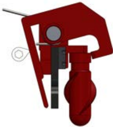
(c) Cam after it has lifted the dropper restraining bar to its maximum deflection
