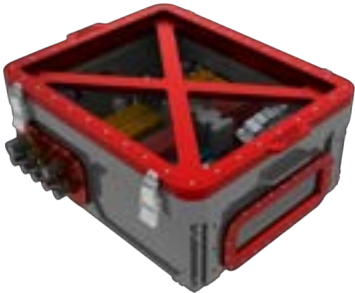
Fig 1. Sirius Upper Hull Pressure Vessel.
