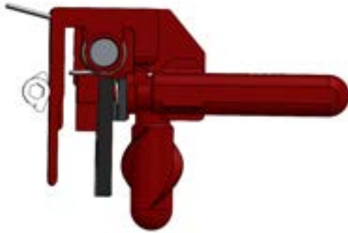
(a) Cam before it has engaged with the Torpedo Restraining Finger
