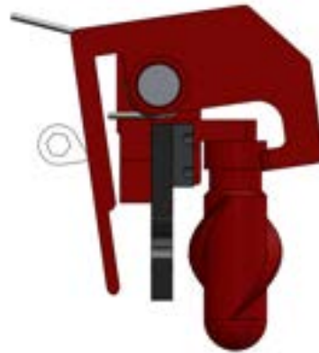
(b) Cam after it has started engaging with the Dropper Restraining Finger
