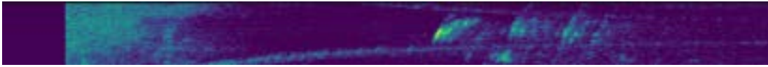
Fig. 43: Original sonar sweep data of a flat panel perpendicular to the robot underwater. The panel can be seen as the first light green blob in the image. The following darker green blobs are acoustic reflections.
