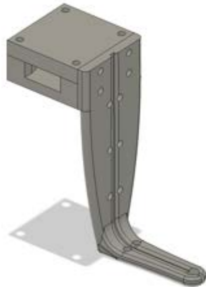
Fig. 18: Old Hydrohone Mount. Required four different mounting locations.
