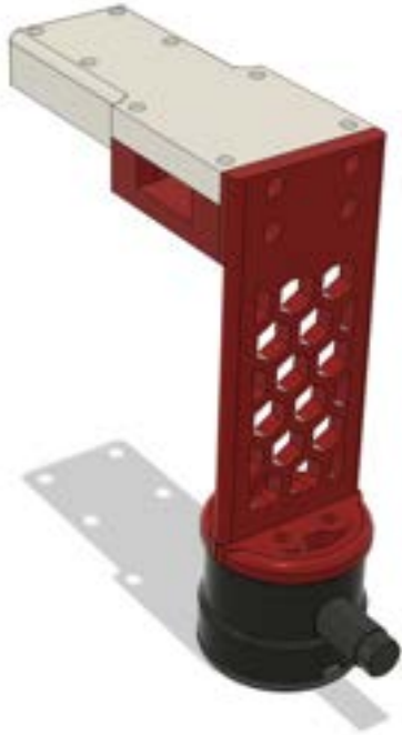
Fig. 20: 1D Sonar Mount. This traded spots with the hydrophone mount a few times when finding the optimum location.
