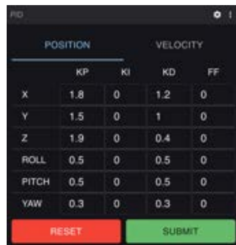
Fig. 37: The PID Panel allows an operator to read and set PID gains. Operators can thus view real-time data using the PID Position Layout (see Fig. 43) and adjust PID constants using the PID Panel to instantly see how they affect Oogway's movement.
