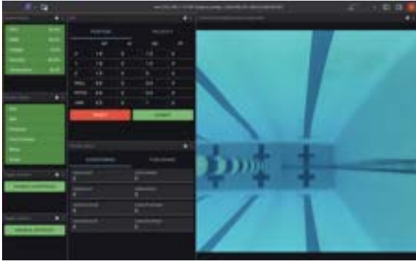
Fig. 32: Standard Foxglove GUI Layout. Our GUI allows us to easily visualize and control Oogway during pool tests. For example, operators can view live bounding boxes, monitor the status of subsystems, and fine-tune PID constants on the fly.
