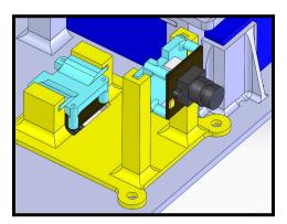
the case that a component needs to be removed, its own individual modular section could be removed without anything being in the way.
