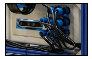
A lot of research took place trying to source ip68 rated passthrough connectors at a reasonable price. Previously, RoboCats had used bluerobotics wire pass-throughs which were great in terms of not leaking, but left a lot to be desired in terms of modularity. After many hours of research we chose the Weipu SP13 series of connectors for their ease of use, cost, and current carrying capabilities.
