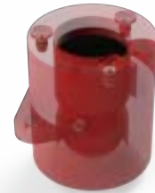
Fig. 7: SeaWolf VIII Dropper enclosure 3D print with the electromagnet stored internally. Design mock-up generated in OnShape.
