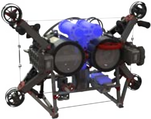
Fig. 2: Rendering of Talos with Buoyancy Additions Highlighted in Blue
