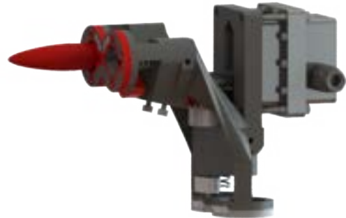
Fig. 1: Redesigned Torpedo Launcher/Marker Dropper Mechanism and Servo Housing
