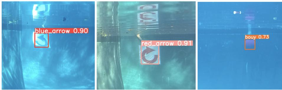
Figure 1.6: YOLOv8 inference on the blue arrow, red arrow, and buoy
