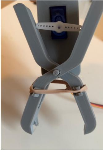
Fig. 6: 3D-printed prototype of the elastically-driven claw design
