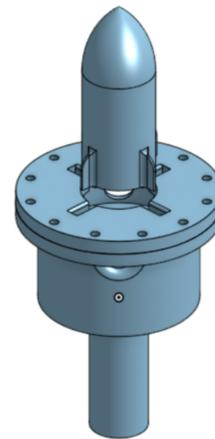
Fig. 9: Launching Torpedo Rotating the shaft aligns the fins with the opening, launching the torpedo
