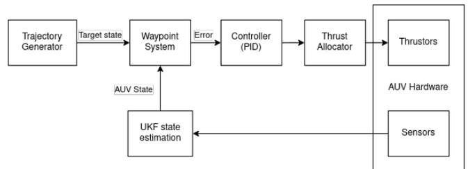
Fig. 11: Block diagram of the software control system used by the Steelhead AUV.
