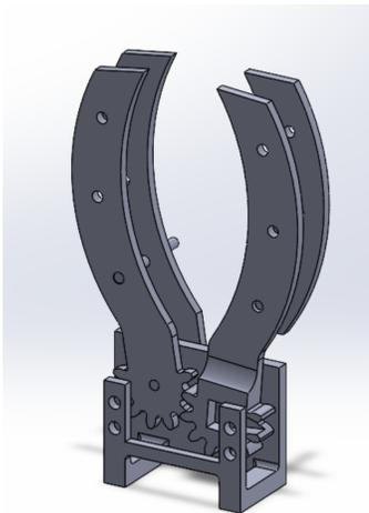
Fig. 7: CAD model of the gear-driven claw design
