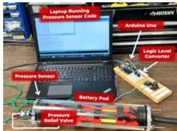
Figure 6: Battery Pod Pressure Testing Rig
