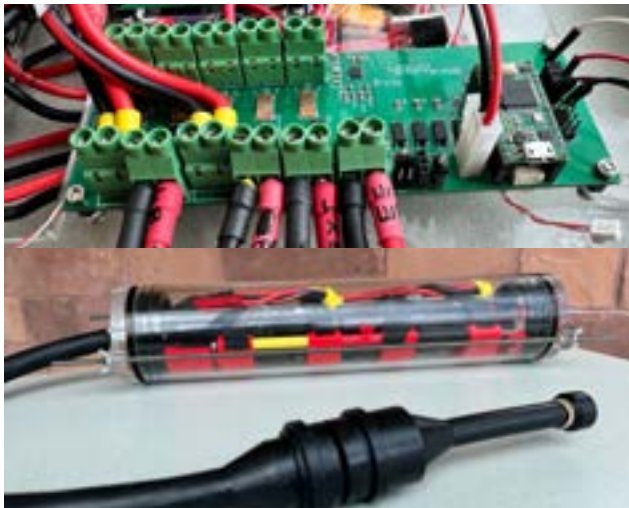
Figure 4: Arctos' Battery Management Board (top), and External Battery Pods (bottom)
