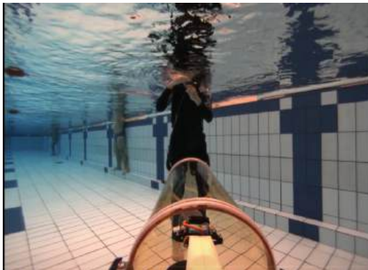
Fig. 45: Testing of a 2 DOF arm with a gripper underwater to benchmark against their research product.
