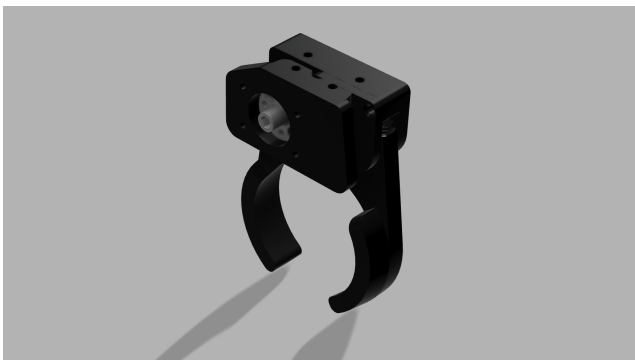
Fig. 2. Rounded grabber fingers tailored to grab the ladle prop
