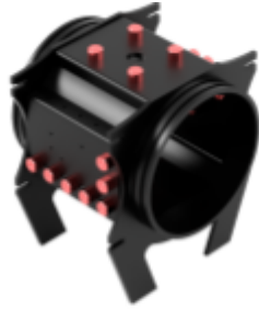
Fig. 3: The central hub with hull penetrators attached.
