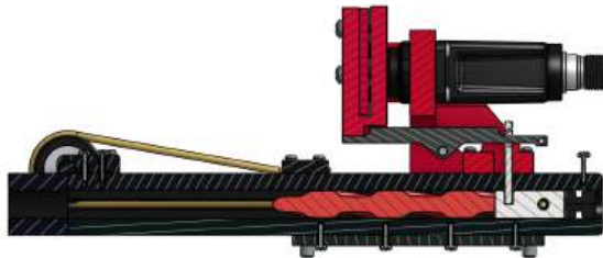
Fig. 7: Cross-section of torpedo launcher chamber with torpedo. Firing block in white, firing mechanism visible above chamber.
