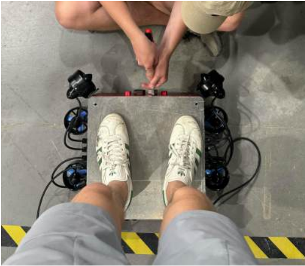
Fig. 18: Pressure test. Note a team member carefully observing the hull for signs of mechanical failure.
