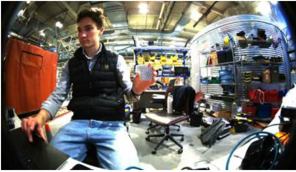
Fig. 17: Testing image sharpness with a focus target.
