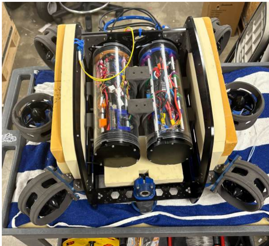
Fig. 25: Crush's Electrical Stack – Populated, Front View
