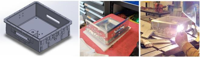
Fig. 2. Hull welding process
