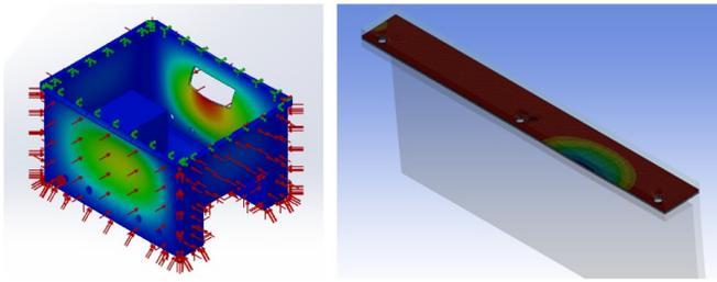
Fig. 1. Simulation results: (a) Hull thickness analysis; (b) Gasket water-tightness analysis.
