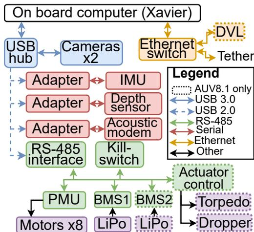
Fig. 3. Simplified architecture of AUV8 and AUVLite
