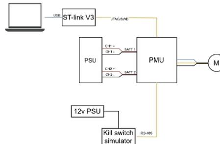
Figure 1: Connection diagram
