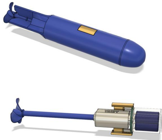
Figures 17 and 18. Torpedo Shell with Internal Motor-Capacitor Assembly
