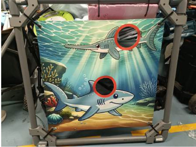
Fig. 16: Torpedo board used for pool tests.
