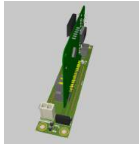
Fig. 9: Individual debug boards that are breadboard compatible.
