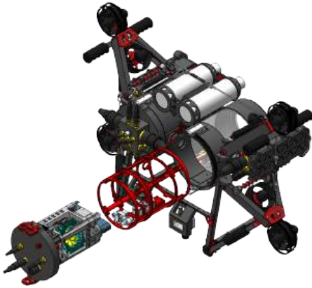
Fig. 3: Exploded CAD assembly of the new rail/cage system
