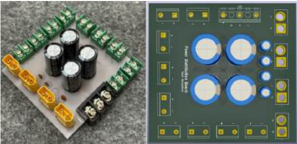
Fig. 10: Power distribution PCB layout and hardware construction for the HAUV
