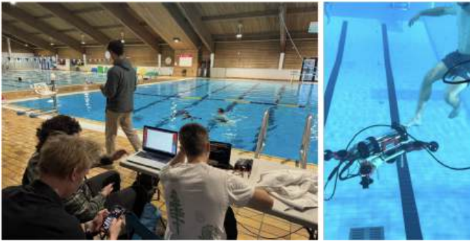
Fig. 14. Left: Software team at pool test. Right: Software lead Eryk testing localization and PID by kicking the AUV.
