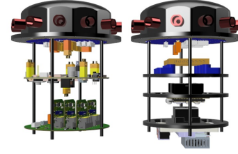
Fig. 3. Electrical Architecture of Peixonauta
