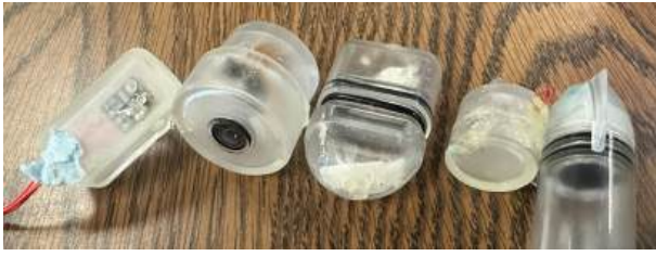
Fig. 9: Torpedo waterproofing panel to test each type of hull-penetrator/opening. From left to right these are testing: the depth sensor and wire sealing, camera sealing, the autonomous torpedo o-rings, wire sealing, and the powered torpedo o-rings.
