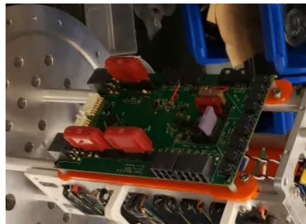
Figure 3: Powerboard mounting configuration
