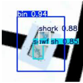
Fig. 11: YOLOv11 bounding boxes on Bins task.
