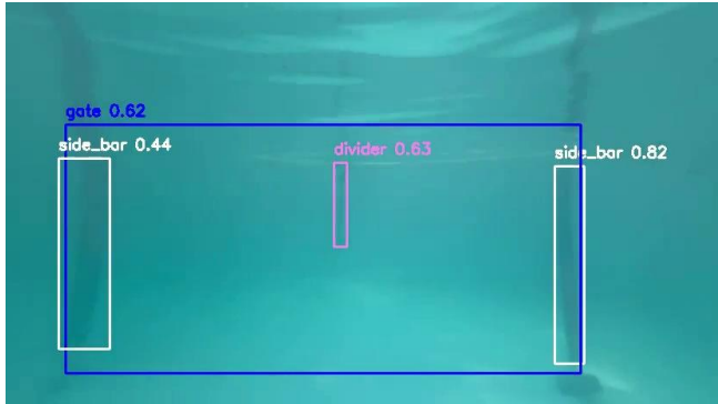
Fig. 05: Mission Gate Detection via AUV Vision System
