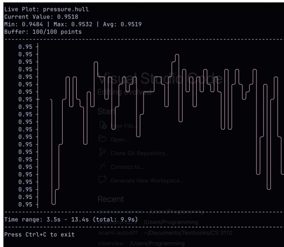
Fig. 25: Example of using shm-plotter to visualize the change in pressure for pressure checks.
