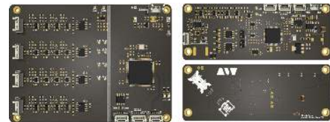
Fig. 10. Pinger Localization and Acoustic Modem Board.
