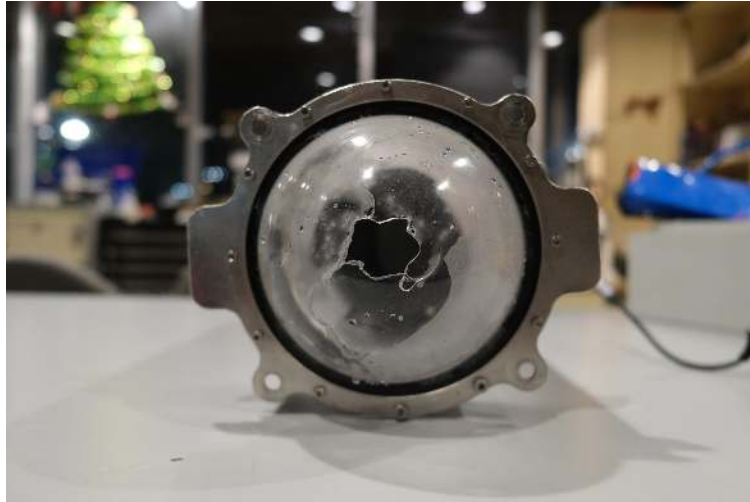
Fig. 24. Deformed dome component observed after high-pressure testing.
