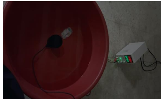
Fig. A7: Experimental setup for real-time acoustic data acquisition using the Ping360 sonar sensor in a controlled water environment
