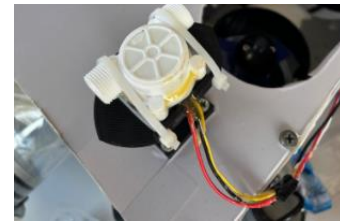
Fig. 2: Flow measurement-based DVL alternative navigation sensor unit.
