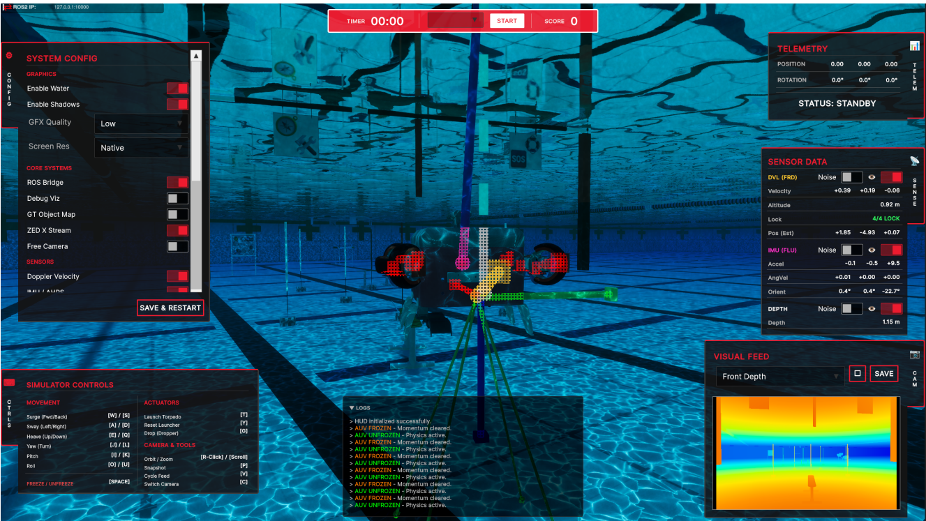
Fig. 39. Unity-based Hardware-in-the-Loop simulation environment used for virtual algorithm validation and mission testing.
