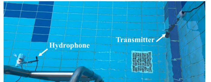
Fig. 8: Validation of Acoustics Comms in the swimming pool
