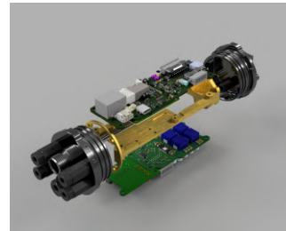
Fig. 3: Render of Bumblebee’s custom software-defined modem stack.
