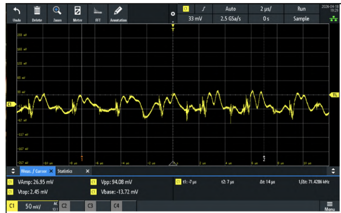
Fig. 31: Sonar power channel voltage ripples under full load and full thrusters
