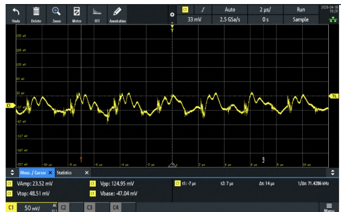
Fig. 28: Sonar power channel with full load (2.7 A, Vpp = 124 mV)
