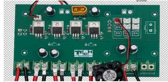
Fig. 8: Power Distribution PCB construction.
