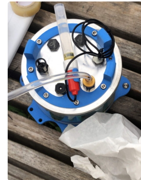
Fig. 38. Pressure testing research module
