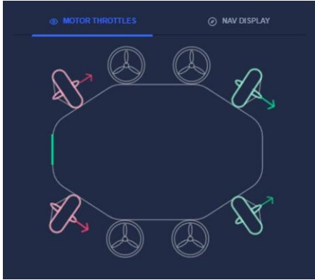
Figure 2 – Thruster Configuration and 6-DOF Motion (Dashboard)
