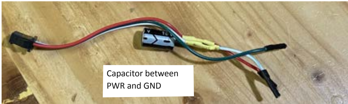
LED Driver Wiring Harness
