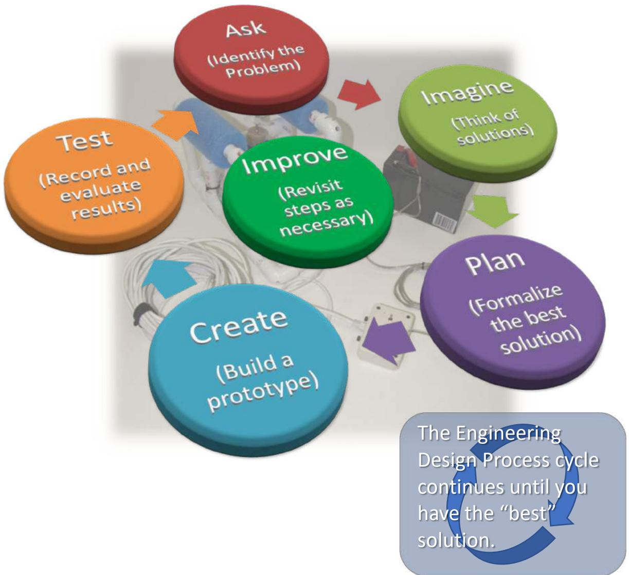
The Engineering Design Process is a repeating set of steps used to solve engineering problems and projects.
