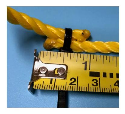
4. Insert the rope through two opposite slots and fasten the ends as shown using an 8" to 10" long cable tie. The ends should overlap 3/4" to 1".
