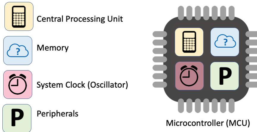
The majority of microcontrollers are embedded in other machinery, such as automobiles, cell phones, appliances, and peripherals for computer systems. Typical peripherals (input and output devices) include switches, relays, solenoids, LED's, and sensors. Microcontrollers normally control a specific task within the device in which they are embedded.
