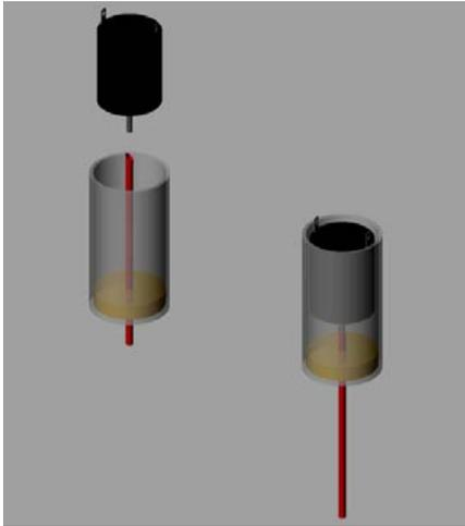
3. Fill one film canister with about ¼” (.5 cm) of hot wax. Carefully place one of your sealed motors in the wax by sticking the motor shaft into the cut end of the straw and continuing to push the motor into the canister, eventually backing the straw all the way out of the can. The motor shaft should now be
