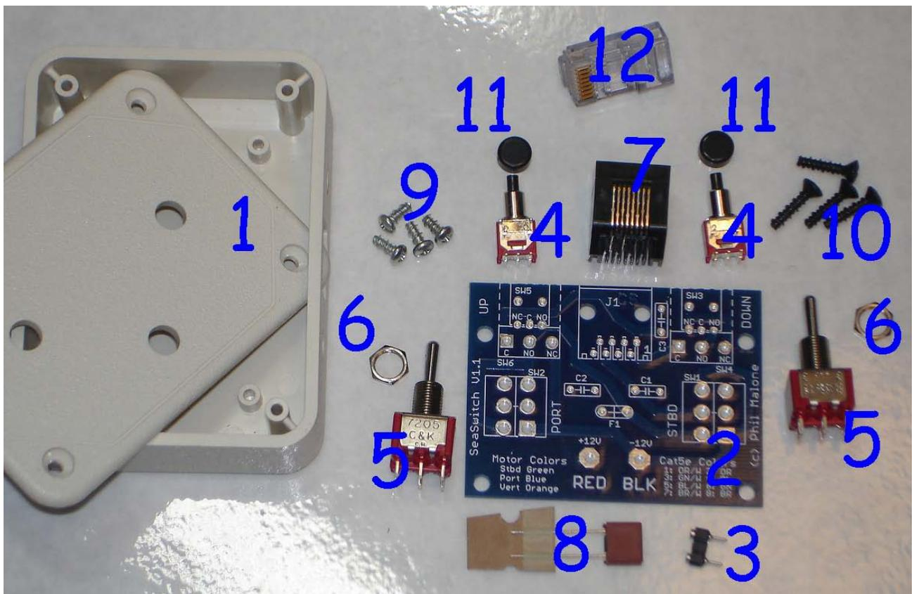
It's important to follow the correct order when adding components to the PCB; otherwise it will be difficult to hold them in place while soldering. Use the sequence below for the easiest assembly. Remember, ALL the parts go on the side of the PCB with the white writing. If you look closely on the back of the board there is a message to help you remember.
