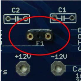
This is the smallest part, and it goes on first, in the middle of the board. The location is labeled F1. Put the socket pins in the two holes, and flip the board over while holding the socket in place.
