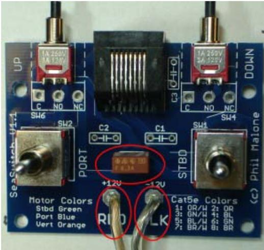
Identify the Positive wire (it may be ridged, or have copper colored wire), and pass it through the hole labeled +12V (RED). Fold it over to hold it in place. Do the same with the other wire through the –12V (BLK) hole. Flip the PCB over, and solder the wires firmly in place. Make sure there aren’t any stray wire strands that may touch and short out. Trim off any excess wire on the boottom of the PCB.
