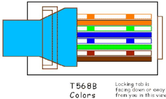
2. Push the wires into the connector with the flat side (side with gold pins) facing up and push them all the way through the connector, until they come out on the other side. The end of the tether cable insulation should be inside the body of the connector, as shown in the above picture. Double check that the wires come out on the other side of the connector in the correct order.
