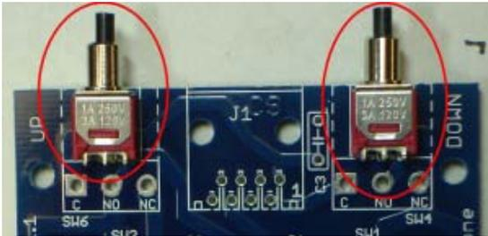
The two push button switches are snapped into their holes at the top of the board. Flip the board over and make sure the PCB is pressed FLAT on the switches while you are soldering these in. If the switches aren't down FLAT, the board won't fit in the box properly.
