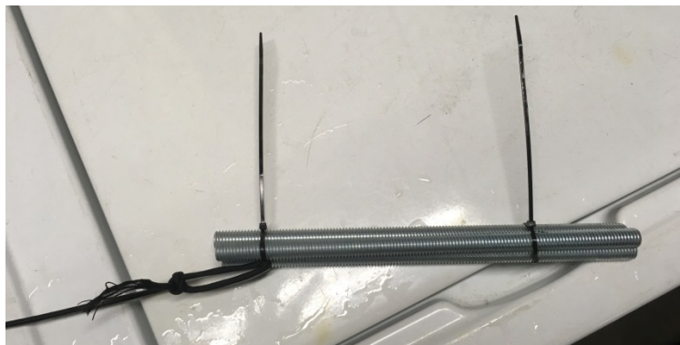
Figure 36 - Threaded rod weights for submerging SeaSense.
