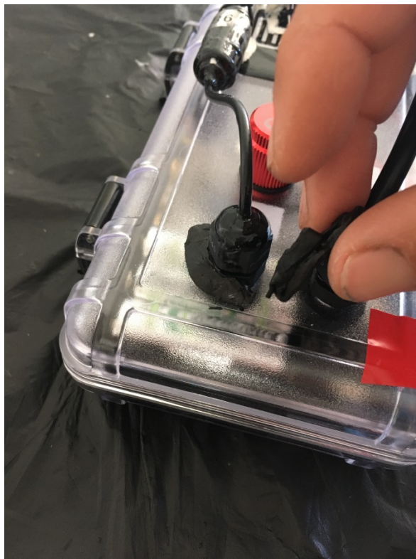
Figure 46 - Temporary leak repair on SeaSense.
