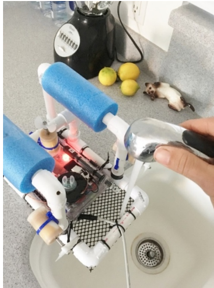
Figure 39 - Rinsing of SeaSense in freshwater.
