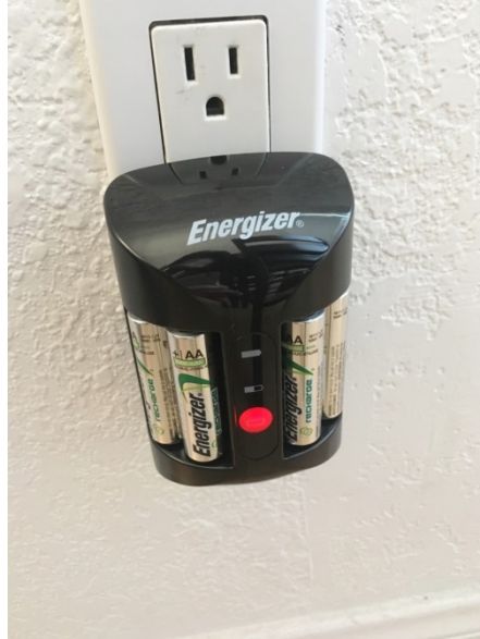
Figure 10 - Battery charge status ( red =charging, orange =nearly done, green =finished).
