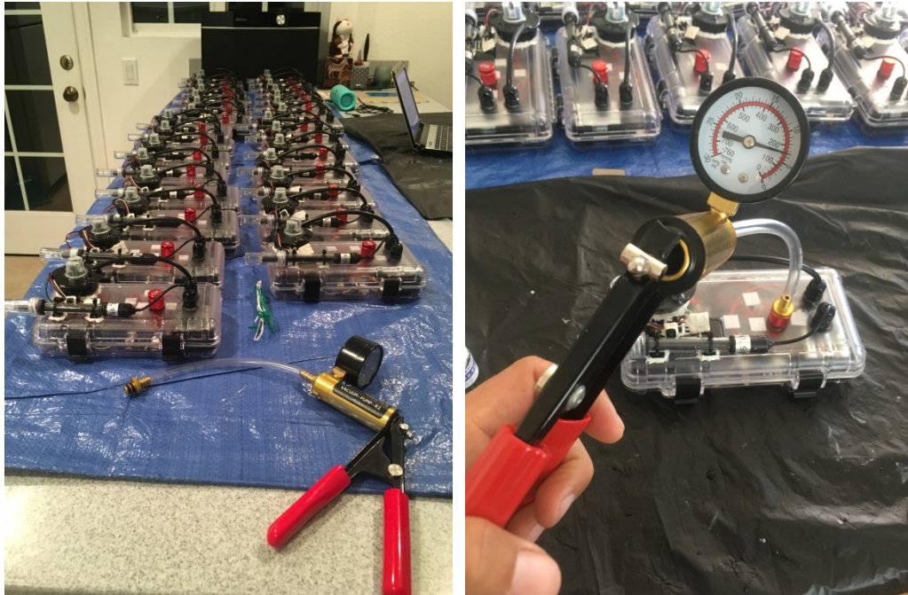
Figure 7 - Vacuum pump for seal check.
