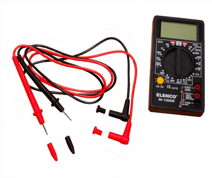
**Name:** Digital Multimeter and Test Probes
