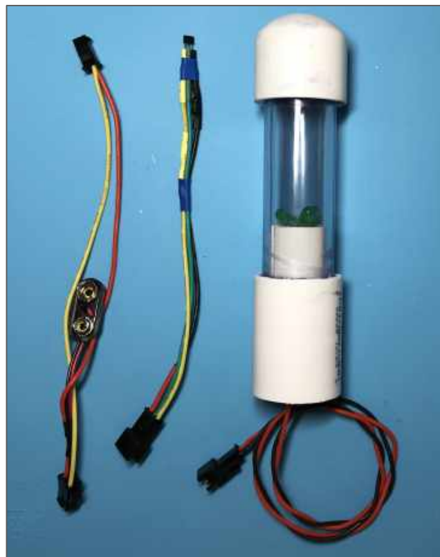
Figure 1.12. Example Using JST Connectors
