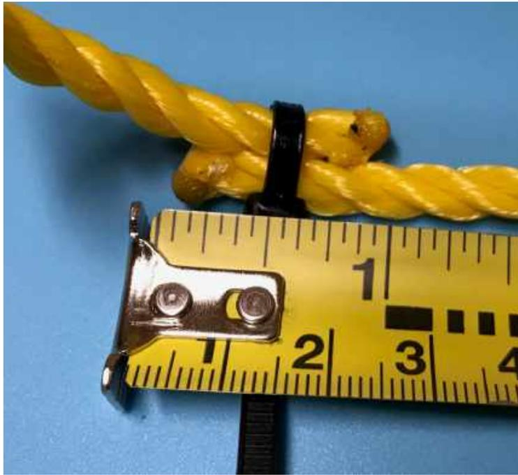
5. Overlap the rope ends 3/4" to 1" and fasten using an 8" to 10" long cable tie.
