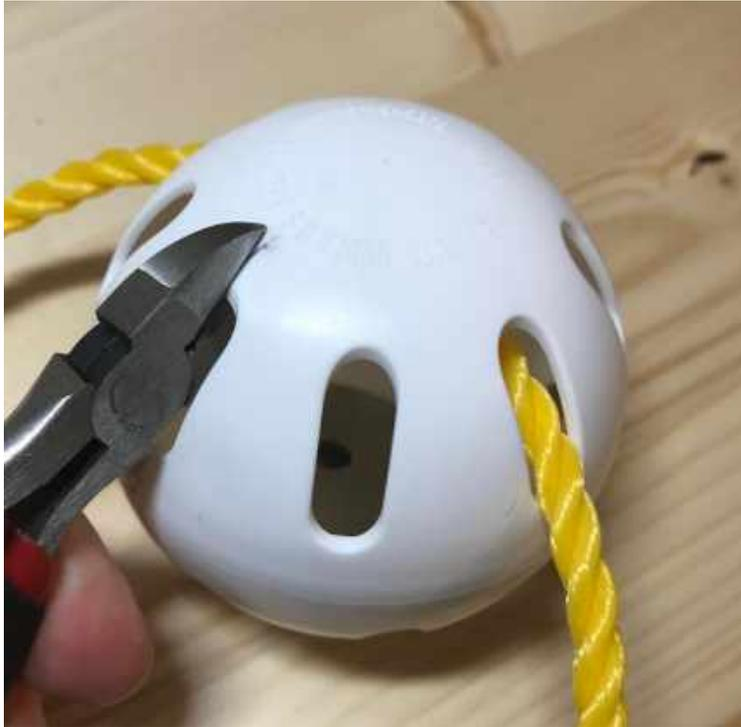
1. Cut a slit on both ends of any slot using diagonal cutting. The slit must be large enough to allow the fender washers to be inserted.
