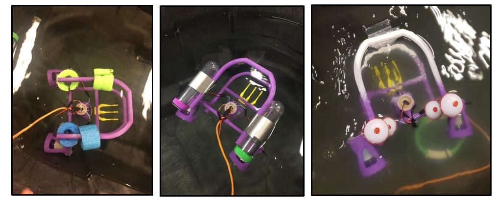
Blue ROV: When we redesigned our ROV, we had to figure out flotation again, but since we knew that flotation needed to be around the motors, figuring out the configuration of the fishing bobbers was very quick.
