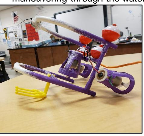
The hook was made with spiked ends so that it could pick up the game piece off the ground and avoid dropping them. As we test-drove it, we realized that the ROV struggled to maintain neutral buoyancy, so we redesigned it to be balanced between the bow and stern.
