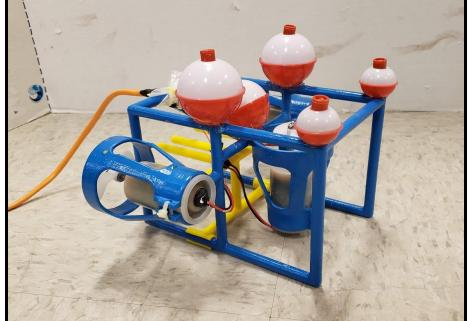
With this rectangular design, the ROV would have greater stability when traveling underwater with the center of mass at the center of the ROV. We also designed the ROV to have a detachable hook that could attach to the vertical bars on the front of the frame.
