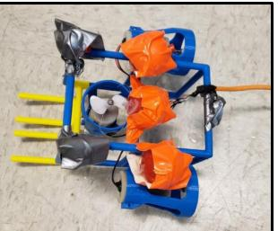
3<sup>rd</sup> hook: On this hook, we made the prongs flatter in hopes of scooping up objects, as well go down to two prongs to ensure the objects were picked up and let go smoothly. At the competition, this hook was very successful in moving objects and was the best of all three designs
