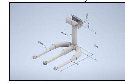
We created this design because we wanted the ROV to porpoise above the water's surface so it could sail higher than the trash and submerge floating trash from the water's surface in one motion. We figured This design would also do well in picking up any sunken pieces of trash because of the detachable hook we had planned to attach on a bar underneath it's center. The thin frame would allow that water to pass through it and increase the ROV's speed and agility when maneuvering through the water.
